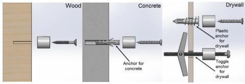
To ensure a secure installation it is important to verify that the mounting area is strong enough to support the weight of the items being mounted, while also supporting the weight of the rod and supports. All installation must be done with proper hardware and correct measures to ensure safety. Make sure to check that the parts are properly installed and secured at the end of each installation. Please follow the below step by step guide for MBS's recommended installation.
