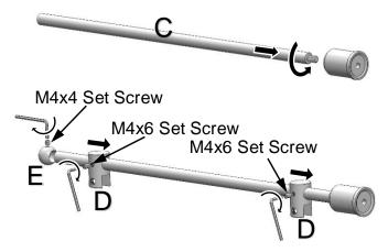
3 Thread Rod Part (C) into Rod support Part (B). Check Stability of the mounted rods. Remove the M4 set screw with a M4 allen key from the panel grips (Part D) and slide them into place on the rod and tighten set screws to keep in place.
