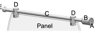
2 Unscrew the rod mount Part (B) from the wall support (Part A). Drop screw through (Part A) and drill to the wall. Once the wall support is firmly placed thread rod mount (Part B) tight onto the wall support (Part A).
