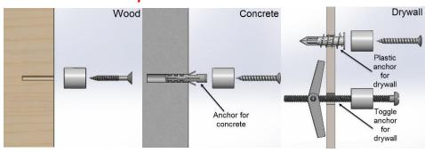
To ensure a secure installation it is important to verify that the mounting area is strong enough to support the weight of the items being mounted, while also supporting the weight of the rod and supports. All installation must be done with proper hardware and correct measures to ensure safety. Make sure to check that the parts are properly installed and secured at the end of each installation. Please follow the below step by step guide for MBS's recommended installation.
