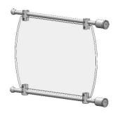
1 Mark the locations where the mounts will be installed. Depending on mounting surface and mounting method pre-drill 1 hole for the anchoring system. Example: Concrete would need 1 pre-drilled 1/4" hole to accept the concrete anchors.
