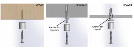
It is essential to check that the top ceiling fixings are strong enough to take the weight of the items being displayed, while allowing for the tension in the cables.. All installation must be done so with proper hardware and protective gears to ensure safety. It is important to check that parts are properly tightened at the end of each installation.
