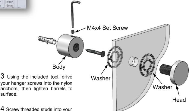
4 Screw threaded studs into your barrels, then place your panel in position and thread on caps until snug.
