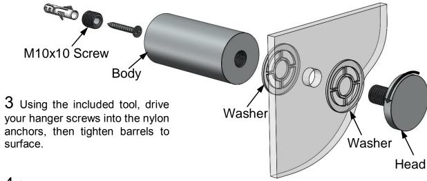
4 Screw threaded studs into your barrels, then place your panel in position and thread on caps until snug.
