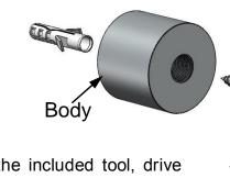
3 Using the included tool, drive your hanger screws into the nylon anchors, then tighten barrels to surface.
