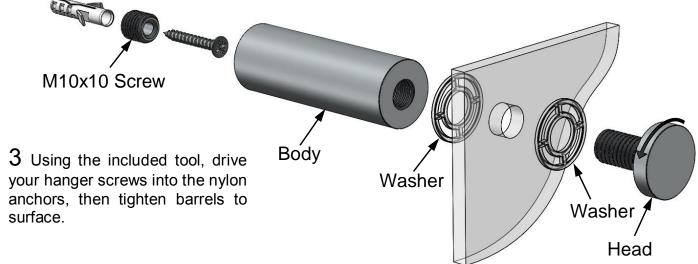
4 Screw threaded studs into your barrels, then place your panel in position and thread on caps until snug.
