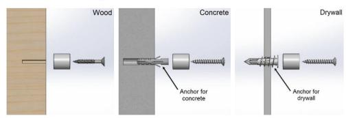
1 Mark the location on the mounting surface where the panel will be installed. Drill any necessary holes.
