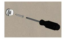
3 Install edge grips on the supports, tighten the M4 set screw closest to the wall.
