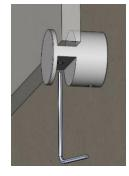
4 Slide the panel all the way through the edge grips and tighten the M4 set screw on the inside edge of the edge grip to secure the panel to the edge grip. Ensure it is a snug fit but it does need to be overtightened.
