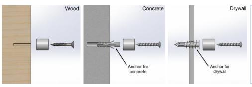
Always check the installation surface to ensure that the substrate will be strong enough to hold the weight of the panel. All installation must be done so with proper hardware and protective gears to ensure safety. It is important to check that parts are properly tightened at the end of each installation.
