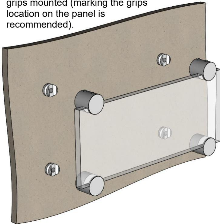
**2** Install the edge grip support found on bottom of edge grip to the wall using mounting hardware.
