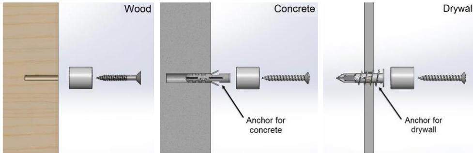
**Always check the installation surface to ensure that the substrate will be strong enough to hold the weight of the panel. All installation must be done so with proper hardware and protective gears to ensure safety. It is important to check that parts are properly tightened at the end of each installation.**
