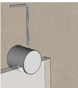
**4** Slide the panel all the way through the edge grips and tighten the M4 set screw on the outside of the edge grip farthest from the wall to secure the panel to the edge grip.
